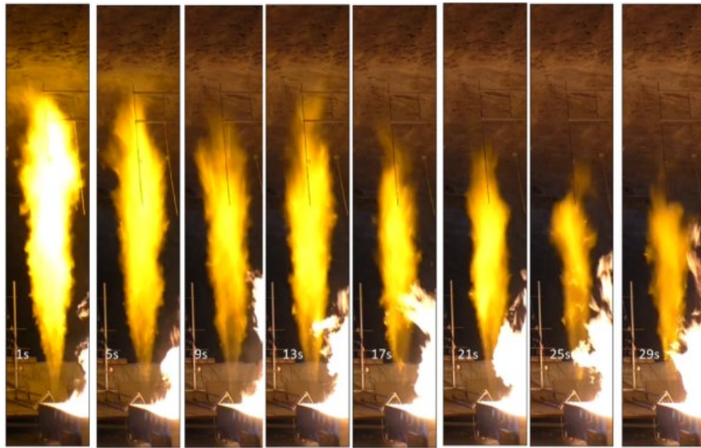
Figure 16. Test 21-15: a) Jet-fire morphology viewed from the rear side, b) Visible flame length with comparison to theory in open environment.
