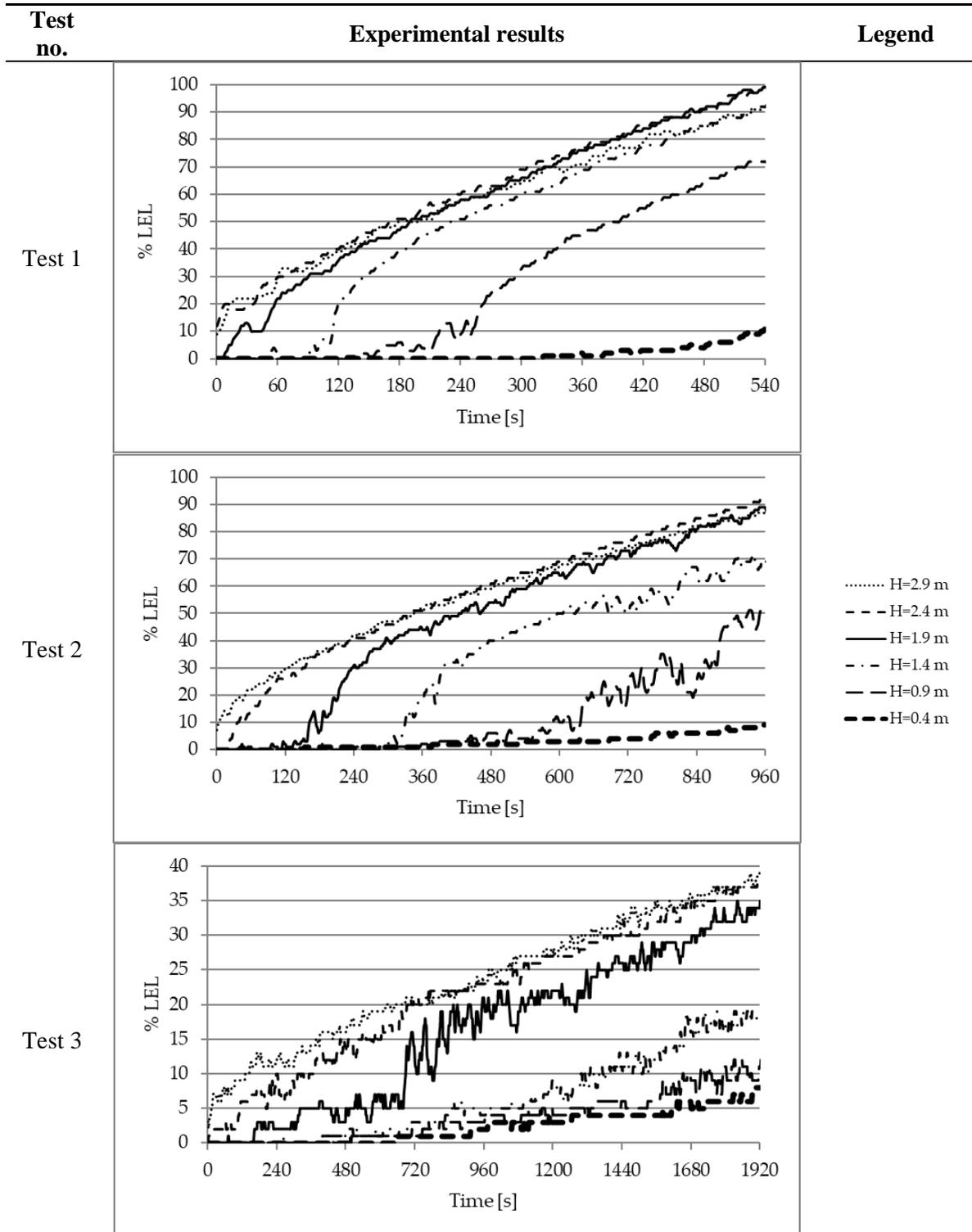
Table 3. Measurement results for hydrogen release from the multi-release point.
