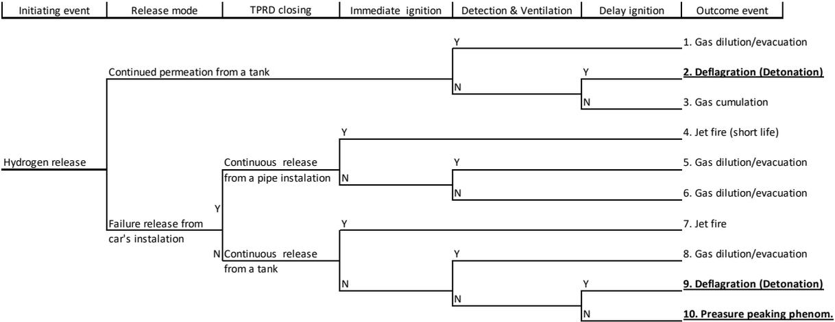
Figure 1. Event tree of hydrogen release incident scenarios
