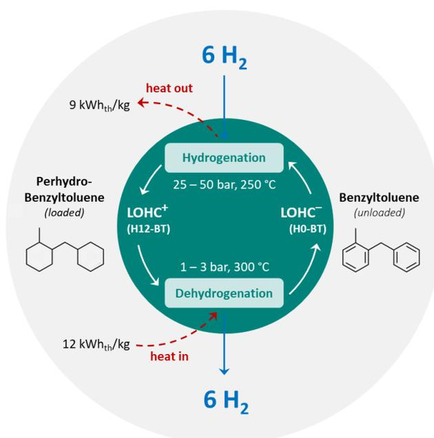
Figure 2. Hydrogen storage and release cycle of the LOHC technology
