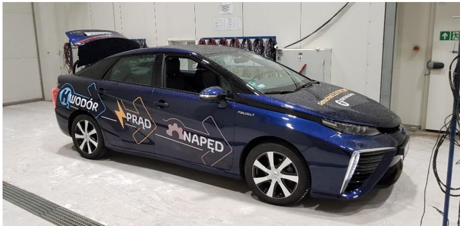
Fig. 1. Toyota Mirai during tests in the thermoclimatic chamber
