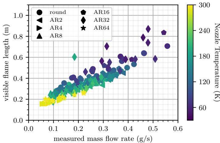
Figure 2. Flame length as a function of mass flow rate
