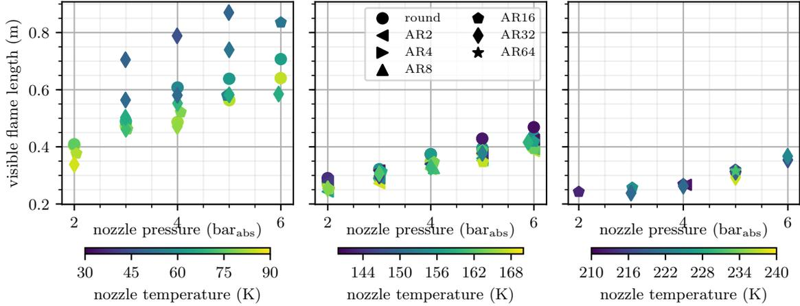
Figure 3. Flame length variation as a function of pressure for several binned temperatures.
