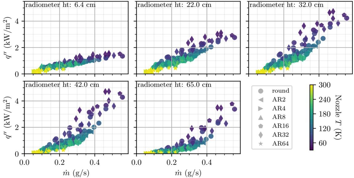
Figure 5. Radiative heat flux measured by each of the radiometers for all test conditions.
