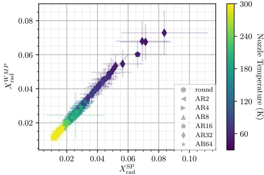
Figure 7. Mean radiant fraction (from all 5 radiometers) calculated using the multi-point vs the single-point method. Errorbars (shown as faint lines in each direction) are the standard deviation of the calculations from the 5 radiometers.
