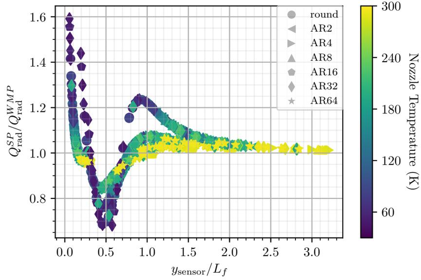
Figure 6. Relative radiant energy calculation using the single-point vs the multi-point method, for all of the five radiometers in this study, as a function of the normalized sensor distance along the flame axis.
