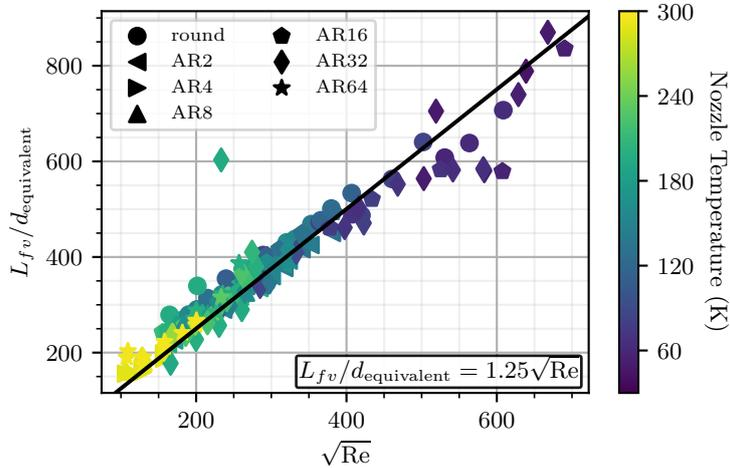
Figure 4. Normalized visible flame length as a function of the square root of the Reynolds number.
