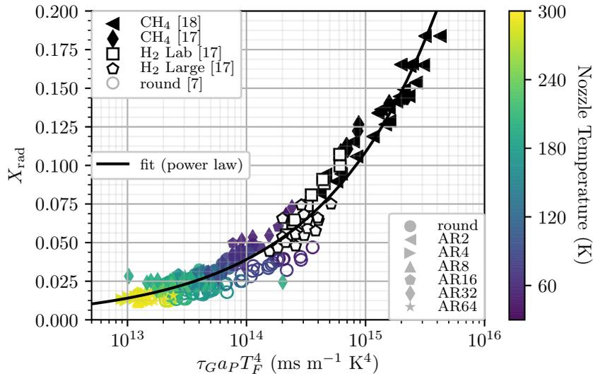
Figure 8. Radiant fraction for cryogenic hydrogen and other literature values for other fuels.
