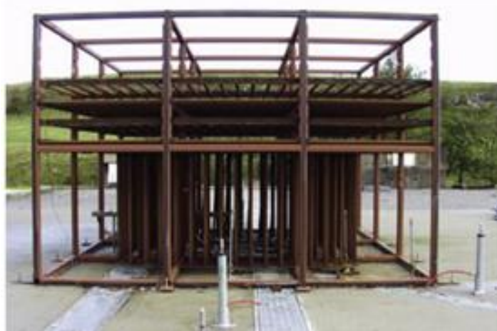
Figure 1. Experimental pipe rig setup with 4-gate configuration [1]
