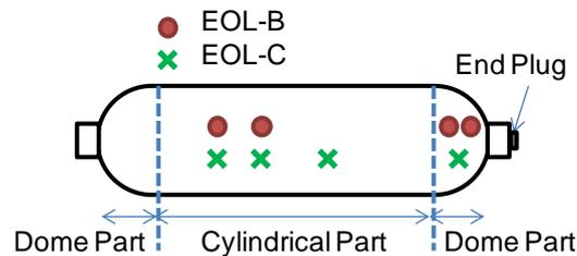
Figure 7 Rupture point of EOL test container
