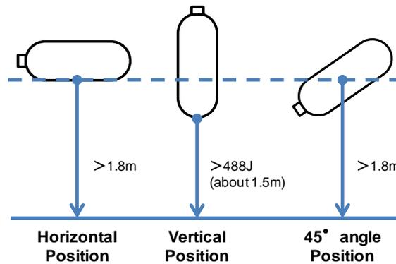
Figure 2 Drop test
