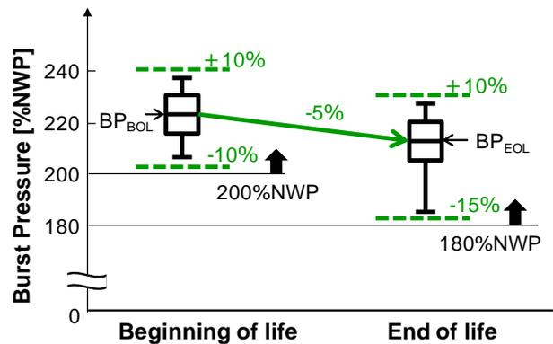
Figure 10 Deterioration of burst pressure between BOL and EOL
