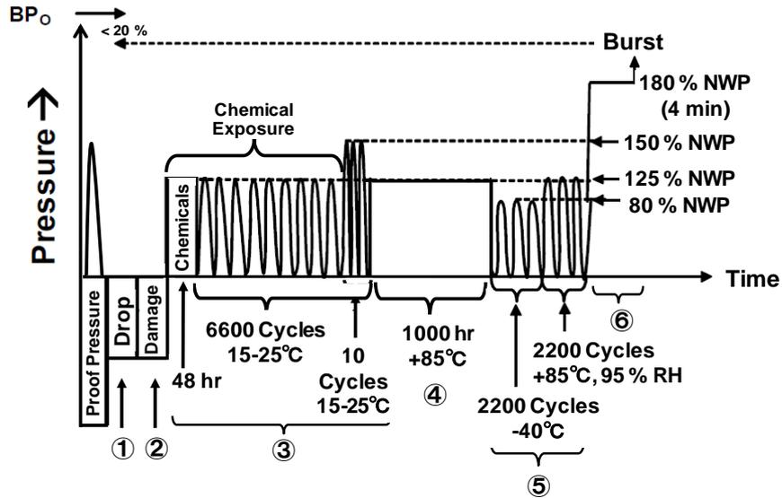
Figure 1 Verification test for performance durability (hydraulic sequential tests)
