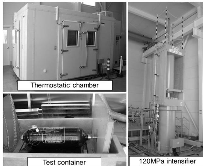
Figure 5 Test apparatus and setting up of test container
