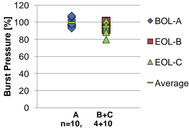
Figure 8 Burst pressure at BOL and EOL
