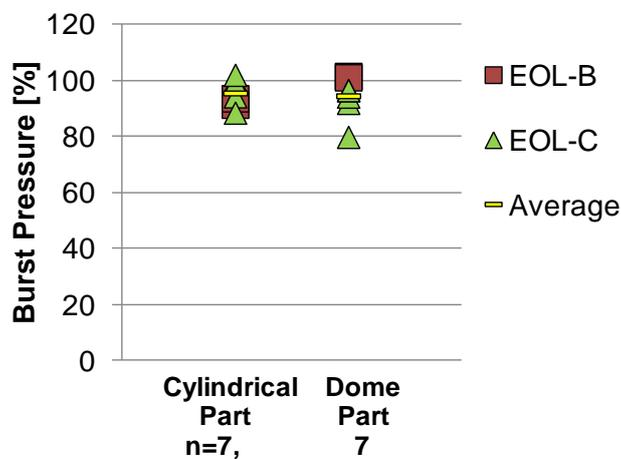
Figure 9 Comparison of burst pressure by rupture point
