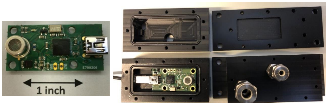
Figure 4: Left: A commercial thermo-conductivity hydrogen sensor. This sensor has been incorporated into the NREL FCEV Exhaust Analyzer. Right: A low-dead volume, custom built hermetically-sealed housing that includes a gas tight electrical feedthrough for the sensor for power and to allow data collection.
