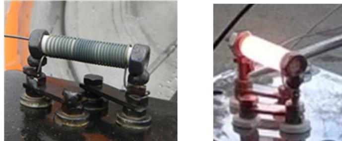
Figure 4 : hot coil arrangement (0.7 m nichrome wire 0.0008 diameter spiralled over a 9 mm diameter 30 mm long alumina cylinder) – electrically heated
