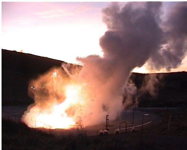
Figure 5. Camera still of ignited hydrogen cloud
