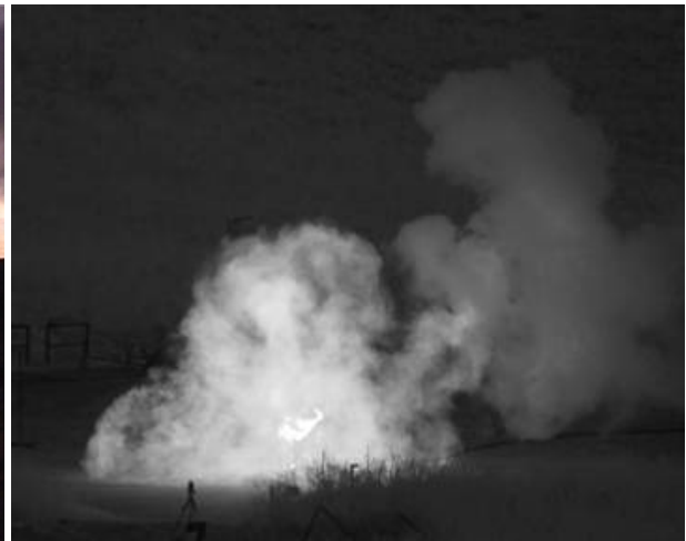
Figure 6. IR still of ignited hydrogen cloud
