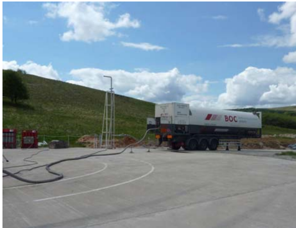
Figure 2. LH2 tanker, vacuum line and vent stack
