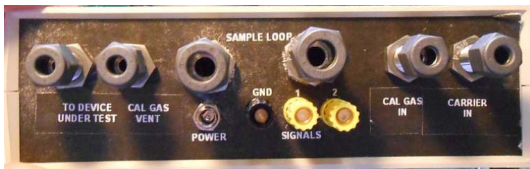
Figure 4: Front panel of the Model 1050 Gas Pulser, used to generate test gas pulses of precisely known duration. (photo used with permission)
