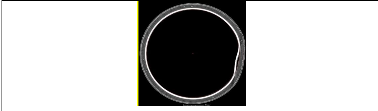
Figure 6. deformation of a metallic liner after subjected to a mechanical impact on the external surface of the COPV.
