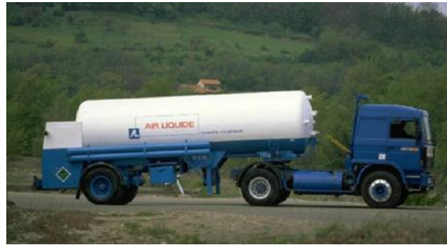
Figure 8. Illustration of a double jacket storage and of a cryogenic trailer
