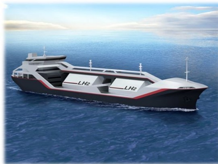
Figure 2. Liquefied hydrogen tanker (Pioneer Ship) (provided by Kawasaki Heavy Industries, Ltd.)
