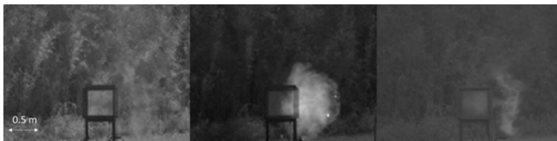
(a) \text{H}_2 \phi=0.5 , burst at 246 kPa (b) \text{H}_2 \phi=2.5 , burst at 183 kPa (c) \text{CH}_4 \phi=1.0 , burst at 264 kPa Figure 3. Flame behavior 5 ms after one wall of vessel burst.
