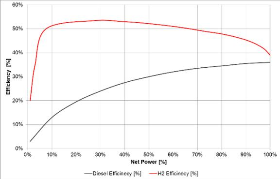
Figure 1a. Diesel ICE vs. FC efficiency.
