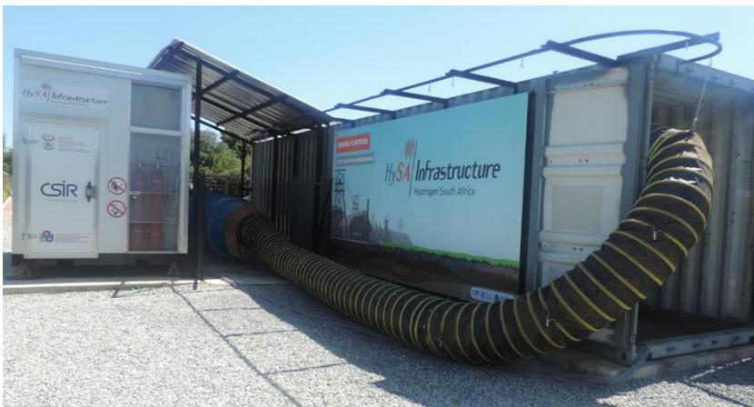
Figure 7 (a). Temporary ventilation test facility.
