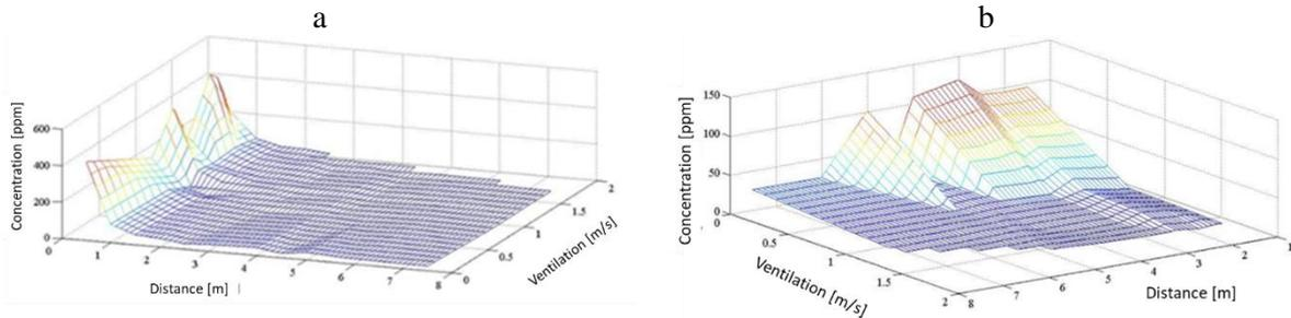
Figure 11. Avg. PPM at release level (a) and 1 meter above release level (b).
