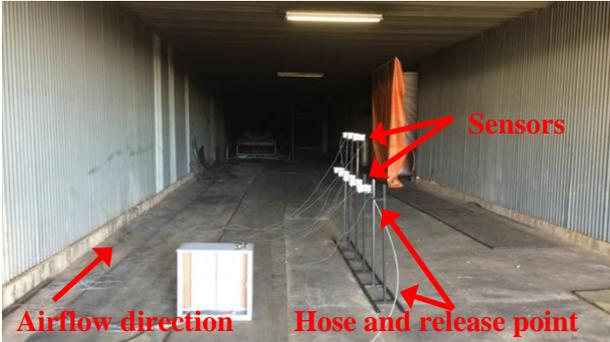
Figure 6 (b). Sensor configuration inside Kloppersbos tunnel.
