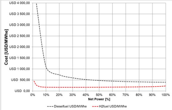
Figure 1b. Diesel vs. hydrogen energy cost.
