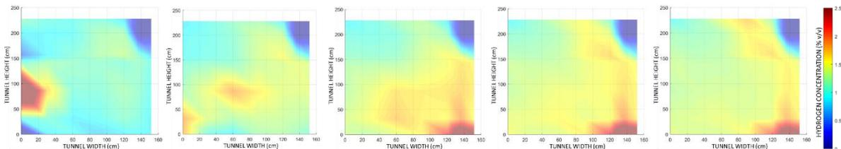
Fig 12. 20 bar, 0.8 mm orifice at 1 m , 2 m, 3 m, 4 m and 5 m.
