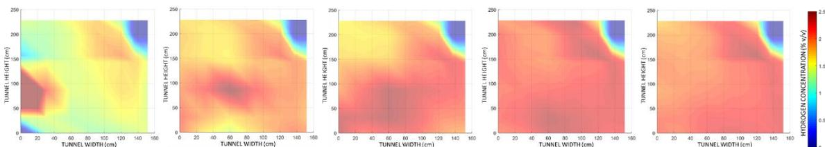
Fig 13. 50 bar, 0.8 mm orifice at 1 m, 2 m, 3 m, 4 m and 5 m.
