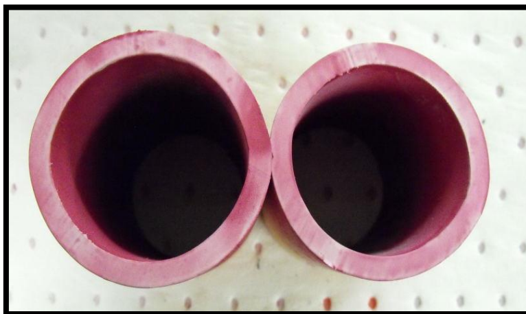
Figure 6 : Sectioned view of hydrogen PE pipe 16413 following hydrostatic testing
