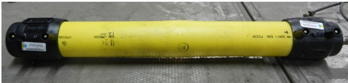
Figure 5 : PE80 pipe prepared for hydrostatic testing
