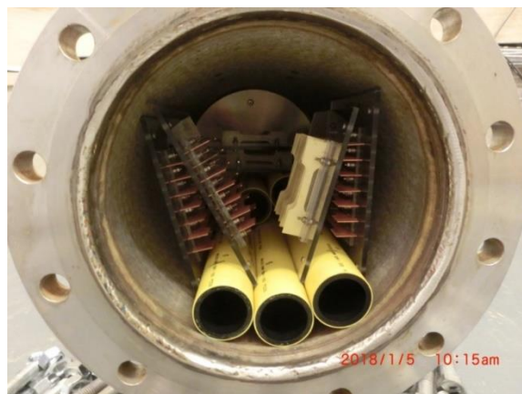
Figure 1 : Samples Within the Gas Soaking Facility Prior to Sealing
