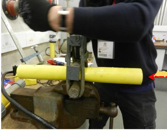
External view of pipe with squeeze-off tool
