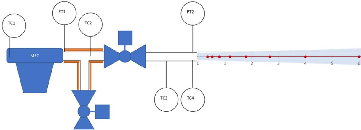
Figure 2: Illustration of the HSL LH2 Release Apparatus along with a proposed Sample Point distribution for the NREL HyWAM in line with the horizontal LH2 release (8 of 32 points).
