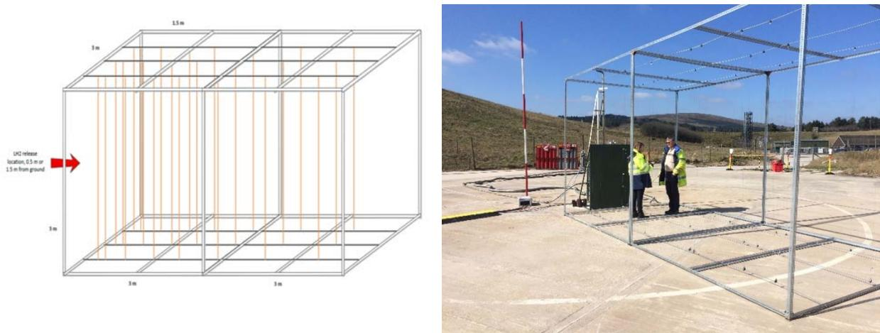
Figure 4: (Left) Open-frame support structure for the NREL HyWAM to support and position sensors and sampling points on vertical support droplines (orange lines). The frame is based upon slotted angle steel strip construction (Dexion). (Right) The fully assembled support structure (3 m by 3 m by 6 m) looking towards the release point (the release hardware is installed behind the green barrier).
