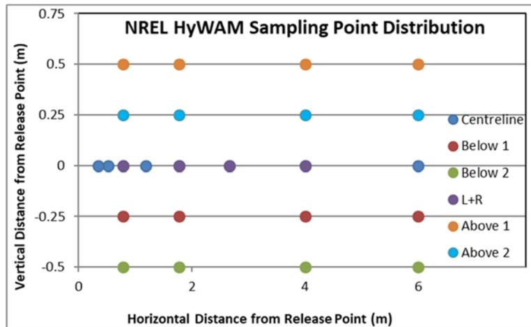
Figure 5: Consensus sample point distribution that is to be implemented for the NREL HyWAM Modules I through IV for the initial horizontal WP3 releases. The sample point distribution may be adjusted based upon field observations and conditions. Up to 32 thermocouples will be co-located with selected Gas Sampling Points.
