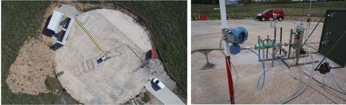
Figure 1: (Left) Aerial view of the test site for the HSL LH<sub>2</sub> release study. (Right) Release station with mass flow meter. For the LH<sub>2</sub> PRESLHY releases, the test site has been updated with an operations building positioned just off the pad and protected by a barrier wall between the pad and control building. Another upgrade has been a frame support structure designed to accommodate gas sampling points for the NREL HyWAM.
