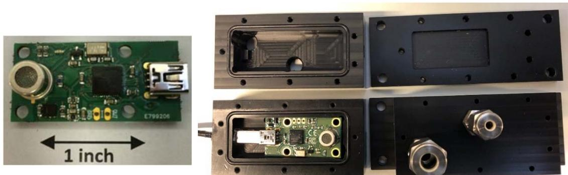
Figure 3: (Left) The commercial thermo-conductivity hydrogen sensor selected for use in the NREL HyWAM. (Right) A low-volume, custom built hermetically-sealed housing that includes a gas tight electrical feedthrough for the sensor USB communication line. Gas flow into and out of the sensor housing is accommodated with two gas-tight fittings for 1/4 inch (outlet) and 1/8 inch (inlet) tubing.
