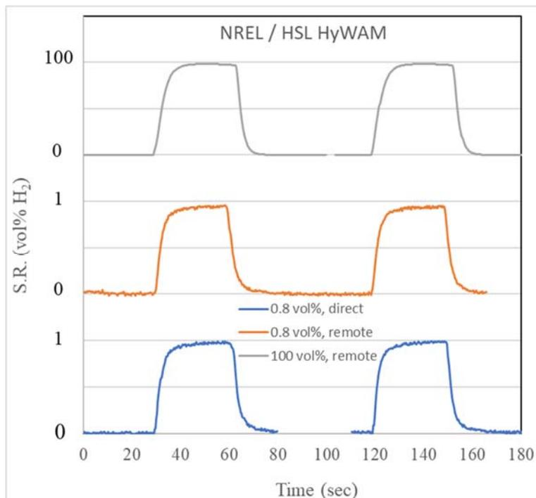
Figure 6: The sensor response (S.R.) to a series of 30-s hydrogen exposures. The sensor was exposed to 0.8 vol% H<sub>2</sub> directly at the sensor housing (—) and through the gas sample line (—). The sensor was also exposed to pure hydrogen (—); the results for pure hydrogen were scaled. There was a time delay of about 10 s for the transport of hydrogen through the pneumatic line, and thus a time correction was used to allow overlaying the data.
