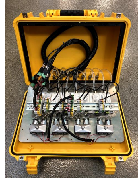
8-Sensor HyWAM module in an environmentally robust enclosure (2021)
