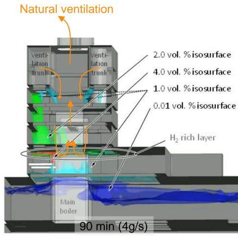
➤ Major source of uncertainty due to unresolved internal structures (piping, walking grids, small components etc.) and entrainment boundary condition.
