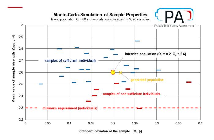
The information about passing the minimum requirement and the mean strength of the batch links the two different worlds of deterministic and probabilistic.
