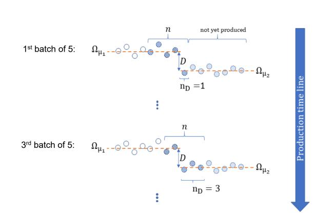
Batch tests target on general faults and not on defective individuals.
