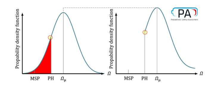
Proof testing sorts the weakest units (red) out and cuts the distribution at the test pressure (density curve). For the moment none can fail at service pressure (MSP), which is a load lower than test pressure (PH).
