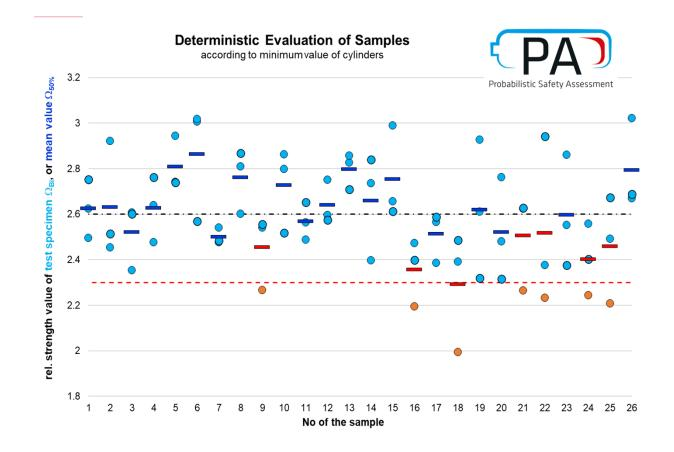
The generated properties of individuals in each sample (here 3) can be checked against a minimum requirement, which allows to count how many batches would not pass.
