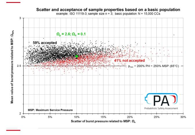
When you ask for a minimum burst pressure on the basis of a small amount of CPVs to be tested there is always a high influence of chance in the test result.
