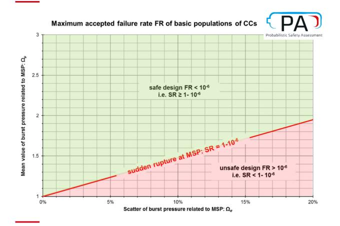
When the data are verified the sample properties (either tested or simulated) need to get checked against the minimum requirement (e.g. 1 of 1 Mio), which depends on the pressurevolume-product (pV).
