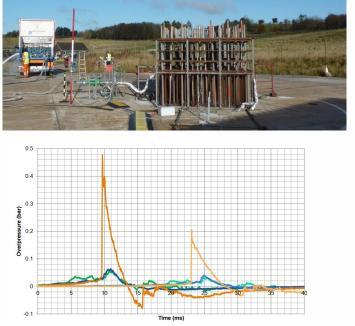
Overpressure comparison for the repeated trials 21 to 23.
