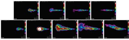
Figure 15: Temperature distribution within jet fire structure. Jet fire radiation for 2-mm nozzle and 10 MPa of initial pressure at T=285 K (upper) and T=80 K.
