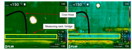
**Figure 6:** Moment of initial flame propagation in hydrogen-air clouds generated by releases of LH2 onto and under water with all measuring equipment at the water basin switched off. The ignition location appears to be somewhere in the cloud at a distance from any physical object. The locations of the release point (cryo hose) and measuring rack/bridge have been indicated.
