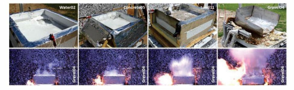
Different degrees of damage to the facility observed in the ignited pool experiments for the different substrates (upper row) and High-Speed video sequence of the final combustion event in experiment Gravel04 (2000 fps, lower row)
