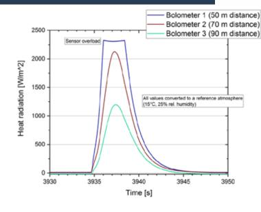
Overpressures measured at 22.5 m and 26.4 m. Heat radiation from the burst of the MLI-insulated vessel.
