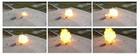
*Figure 11*: Fireball development after the failure of an MLI-insulated vessel positioned horizontally filled with LH2 a seen from an UAV flying over the H2TA
