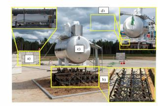
Experimental setup of a MLI-insulated vessel positioned horizontally filled with LH<sub>2</sub>
