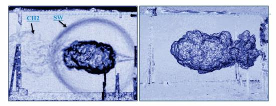
Shock wave formation (left) and a stationary jet fire (right) established following ignition of 4-mm nozzle and 20 MPa CryoH<sub>2</sub>G release: SW –shock wave; CH2 –unignited H<sub>2</sub>
