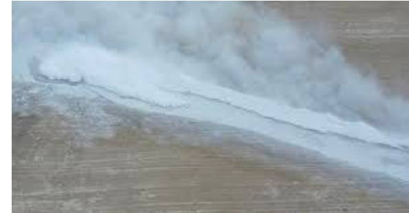
LH2 large-scale release and delayed ignition PRESLHY project - HSE
