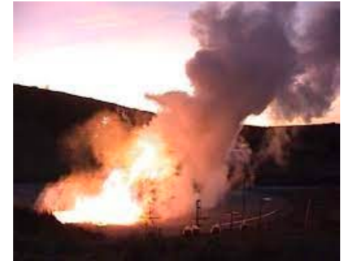
LH2 large-scale release and delayed ignition PRESLHY project - HSE
