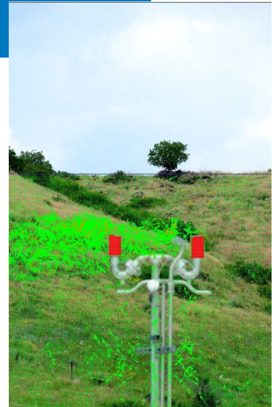
Example of Schlieren observed at a hydrogen vent at NREL.
