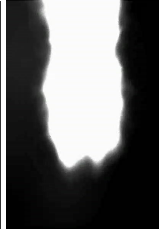
Jet flame is sustained after ignition
