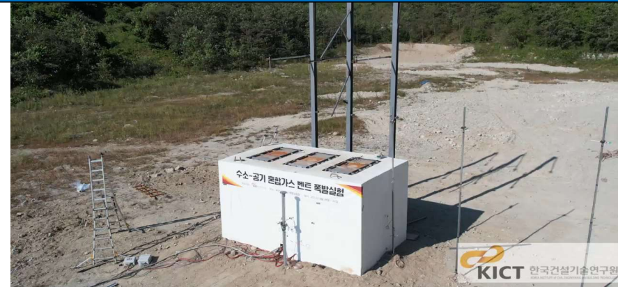
Airtight condition & hydrogen concentration 20%
