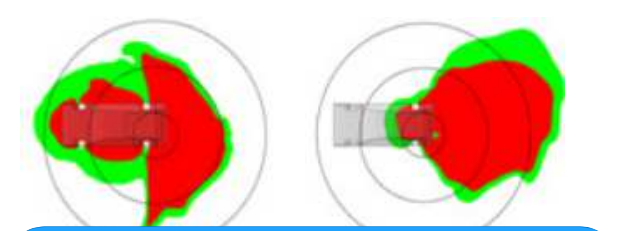
Heat flux profile around the vehicle at different TPRD discharge angles (90°vs45°)
