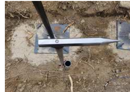
<Incident overpressure transducer>
