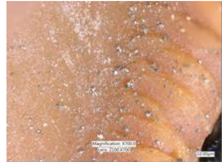
Figure 4. Microscopic image of a failed valve seat showing metal debris
