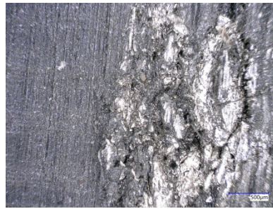
Figure 3. Microscopic image of metal impregnated rider band collected from a compressor after a failure.
