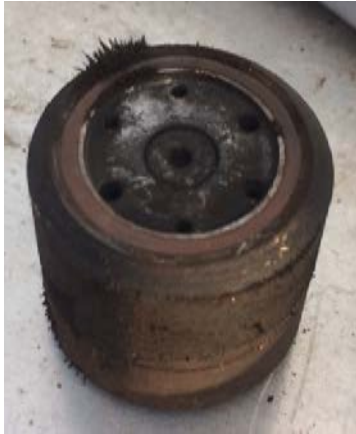
Figure 2. Failed check valve from a leaking compressor. Metallic debris is shown in the top left.
