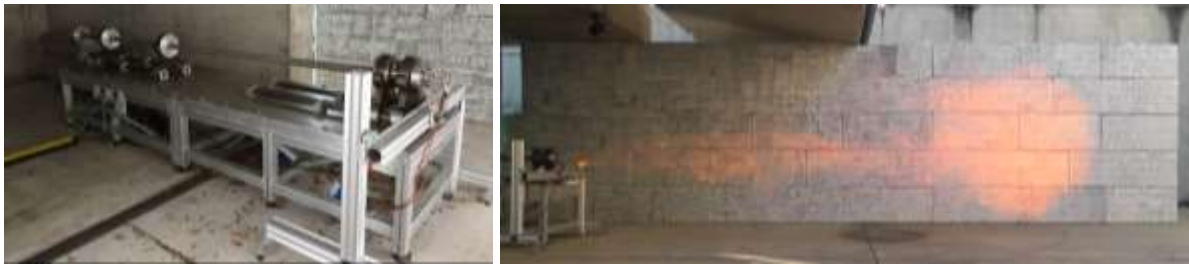
Figure 8 Open air experimental plant building of Fraunhofer ICT to be used for the high pressure storage tube (l.) and the concrete wall, here with an ignited jet in front of it (r.)
