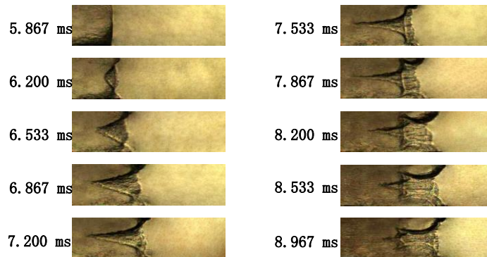
Figure 2. Flame shape changes in channel (b) with \alpha=6.625
