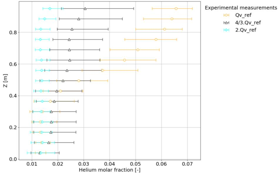
Figure 8. Experimental helium distribution on the height of the 1-m<sup>3</sup> enclosure at steady state according to ventilation flow rate, for 100-NL.min<sup>-1</sup> helium releasing flow rate.
