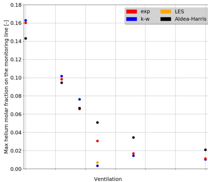
Figure 10. Experimental, numerical and analytical helium maximal concentration at steady state for  $100\text{-NL}\cdot\text{min}^{-1}$  helium releasing flow rate according to ventilation flow rate.
