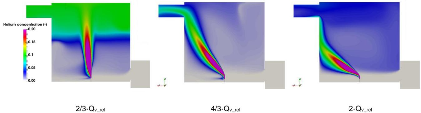
Figure 11. Mechanical ventilation impact on helium jet.
