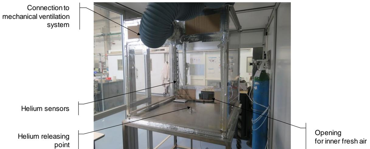
Figure 3. Mechanical ventilation systems.
