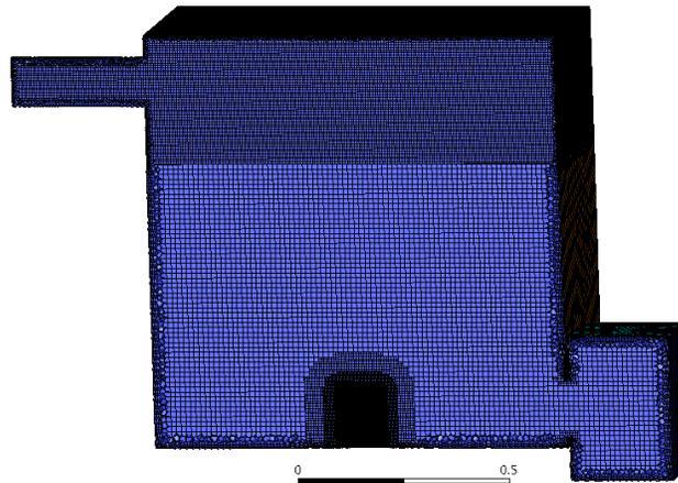
Figure 7. Meshing Hexahedral 1.5 M close to symmetry plane.
