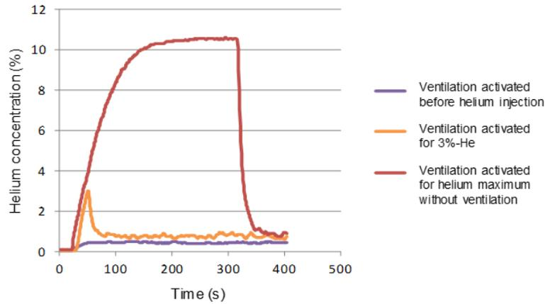
Figure 6. Ventilation activation mode.
