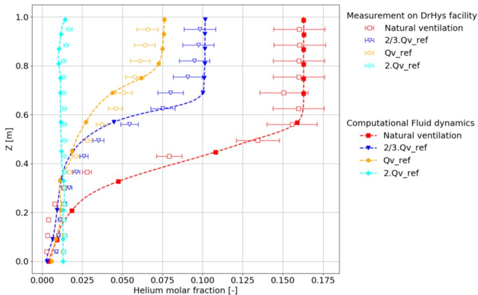
Figure 9. Helium distribution on the height of the  $1\text{-m}^3$  enclosure at steady state according to ventilation flow rate, for  $100\text{-NL}\cdot\text{min}^{-1}$  helium releasing flow rate. Numerical and experimental data.
