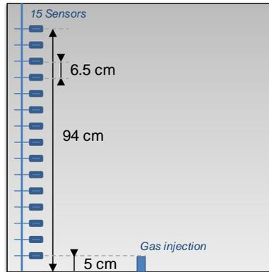
Figure 4. Location of the sensors in the 1-m<sup>3</sup> build-up enclosure.
