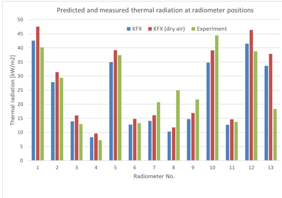
Figure 7. Comparison of predicted and measured thermal radiation at different radiometer locations for Jet Fire No. 2.
