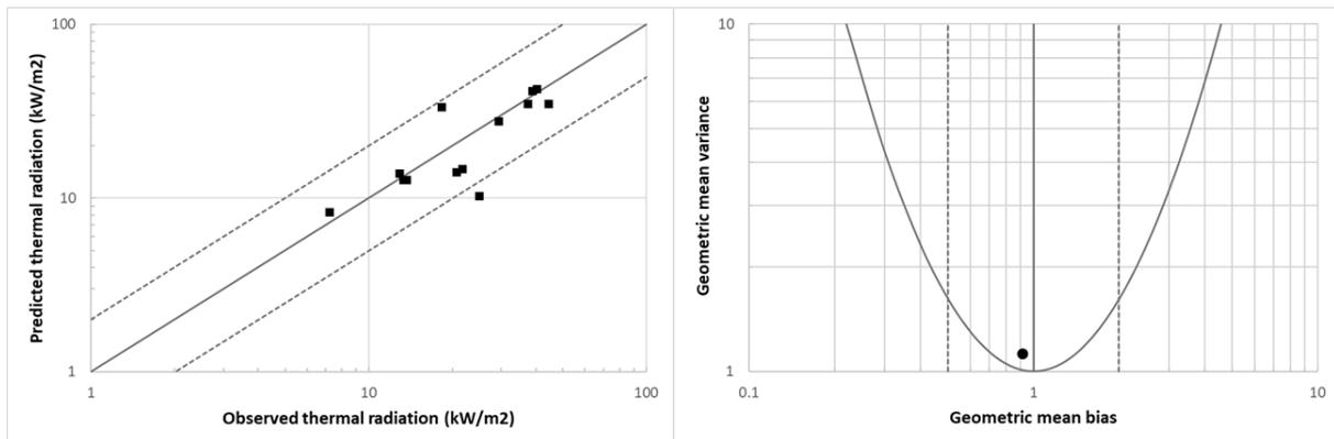
Figure 8. KFX™ model performance for Jet Fire No. 2.
