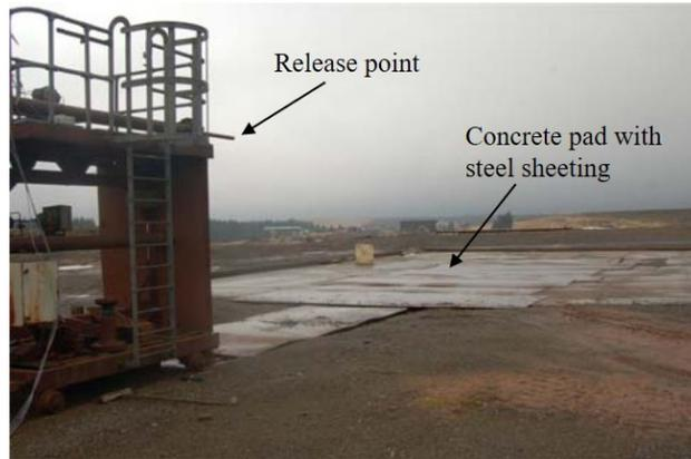
Figure 1. Release setup for the large-scale hydrogen jet fire experiments at the Spadeadam test site (Photo from Ekoto et al. [6]).
