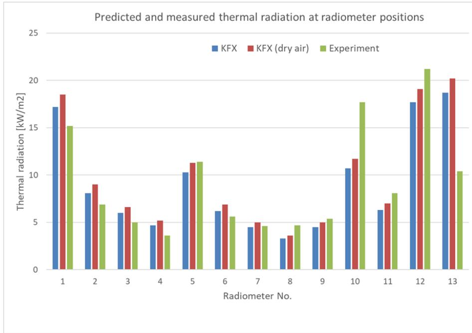
Figure 4. Comparison of predicted and measured thermal radiation at different radiometer locations for Jet Fire No. 1.
