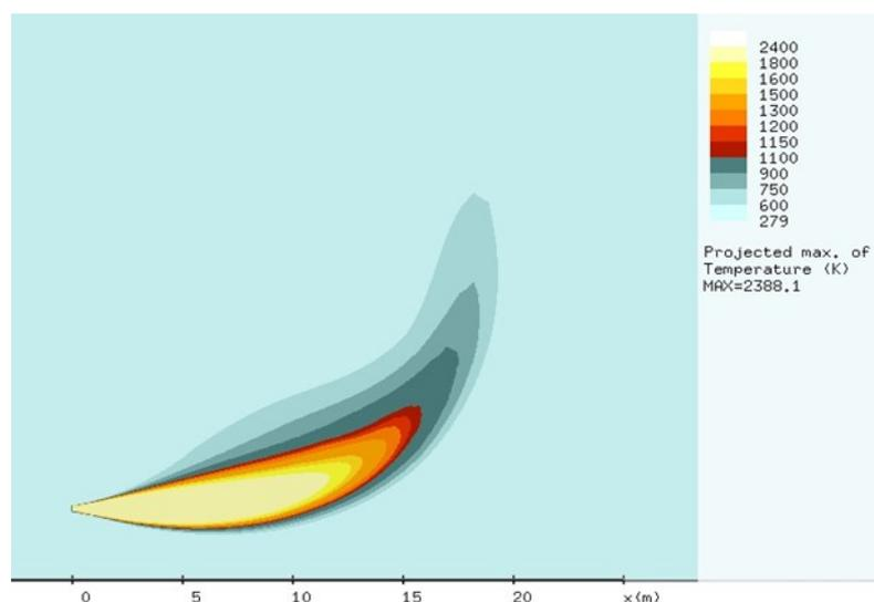
Figure 3. Predicted iso-contours of projected maximum gas temperature for Jet Fire No. 1.
