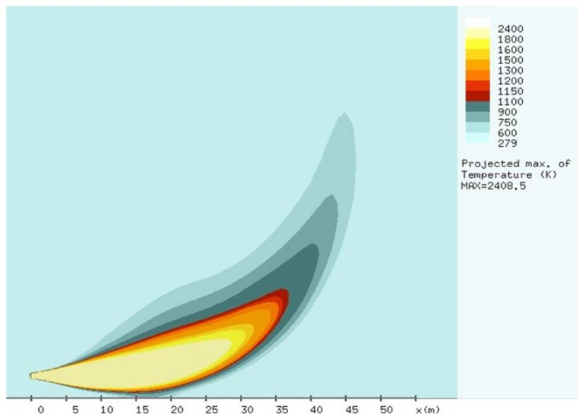
Figure 6. Predicted iso-contours of projected maximum gas temperature for Jet Fire No. 2.
