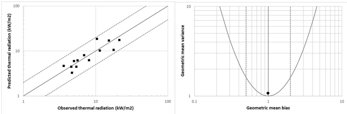
Figure 5. KFX™ model performance for Jet Fire No. 1.
