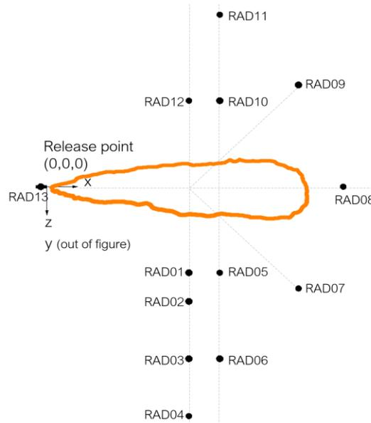
Figure 2. Schematic of the radiometer layout during the hydrogen jet fire experiments.
