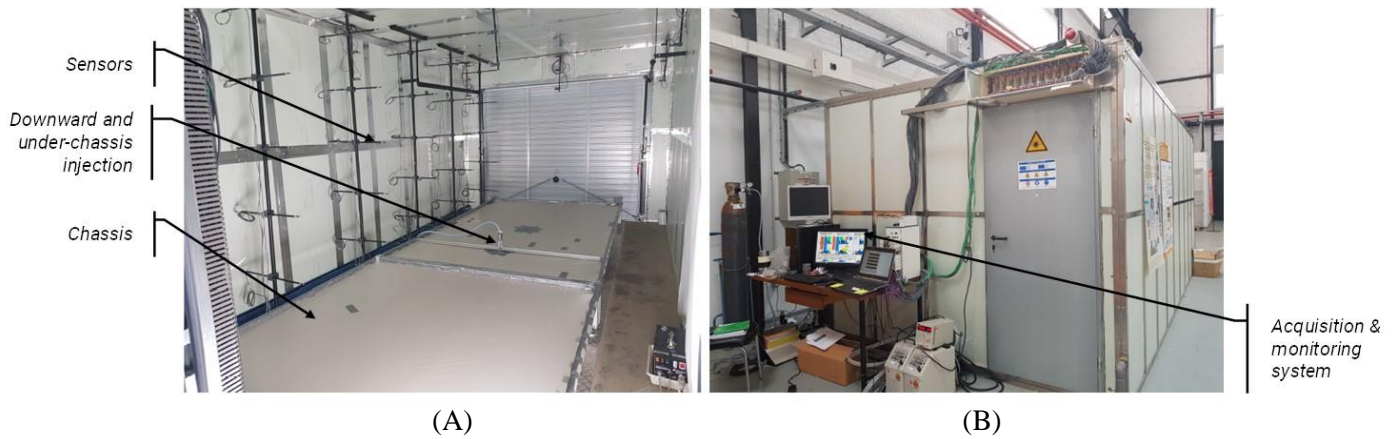
Figure 2. “GARAGE” CEA experimental facility. (A) Inside the enclosure with the chassis in grey close to the roof, (B) outside the enclosure with the sensors monitoring system.
