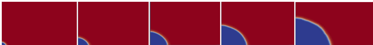
Figure 5: Flame propagation (iso-surface of regress variable, b ) at different times 15 ms, 25 ms, 35 ms, 45 ms and 55 ms (left to right). The results correspond to Case-B for stoichiometric hydrogen concentration. The figure represents one-quarter of the box.
