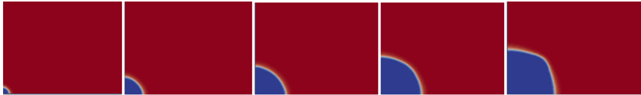
Figure 2: Flame propagation (iso-surface of regress variable, b ) at different times i.e., 15 ms, 25 ms, 35 ms, 45 ms and 55 ms, (left to right), respectively. The results correspond to Case-A (hydrogen concentration 30 %). The figure represents one-quarter of the box.
