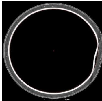
Figure 11. Deformation of a metallic liner after subjected to a mechanical impact on the external surface of the COPV.
