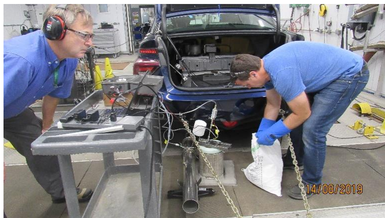
Figure 4: NREL and ECCC team members interfacing the prototype FCEV Exhaust Gas Analyzer to a commercial FCEV
