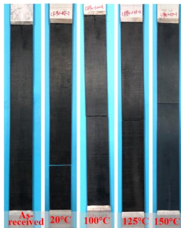
Figure 6. Fracture morphology of CF90 specimen at different heating temperatures.
