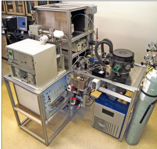
Figure 4: The NREL Safety Sensor Test Apparatus (SSTA) is capable of quantitatively assessing critical sensor metrological performance metrics.
