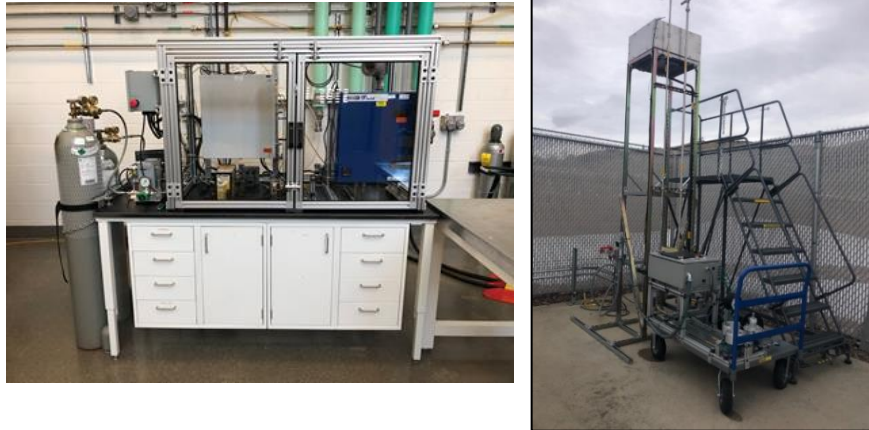
Figure 5: (Left): The Process Gas Sensor Test Apparatus allows sensor testing to pure hydrogen or other flammable gas. It was designed to be compliant to NFPA 70 even when using non-listed instruments and sensors. (Right): The “leak-on-demand” test apparatus allows for the outdoor production of a hydrogen release under controlled conditions and is deployed within HITRF.
