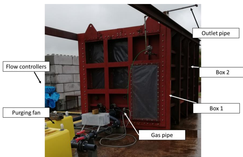
Figure 1. Metallic enclosure for vented deflagrations
