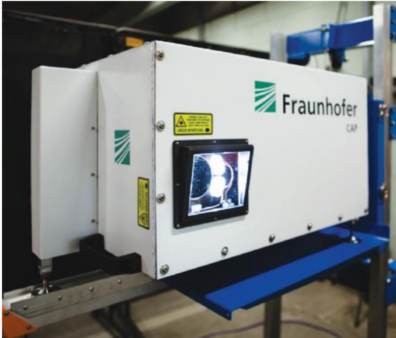
Figure 4. Field deployed hydrogen sensing system.
