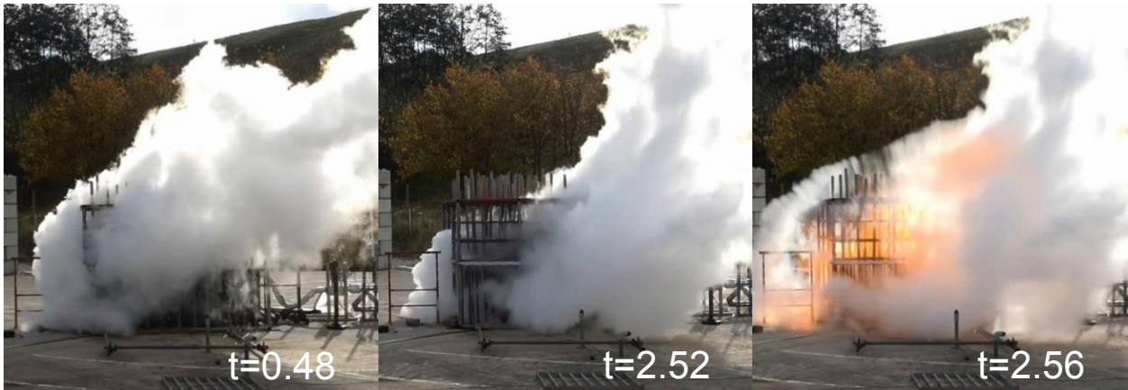
Figure 6. Series of stills showing sudden gust immediately prior to ignition for Test 23.
