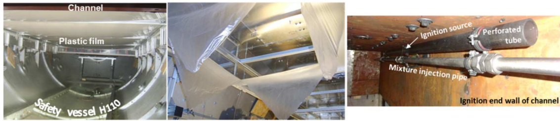
Figure 4. Sealed channel (left), late stage of x-shaped cut of a film segment (center) and ignition device (right).
