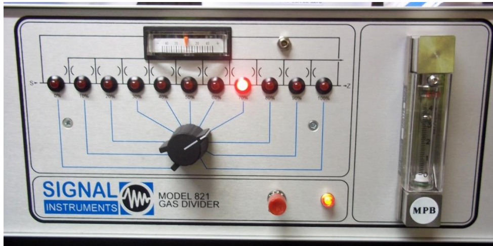
Figure 1. Sigma 821S Gas divider used to control hydrogen concentration at test environment inlet
