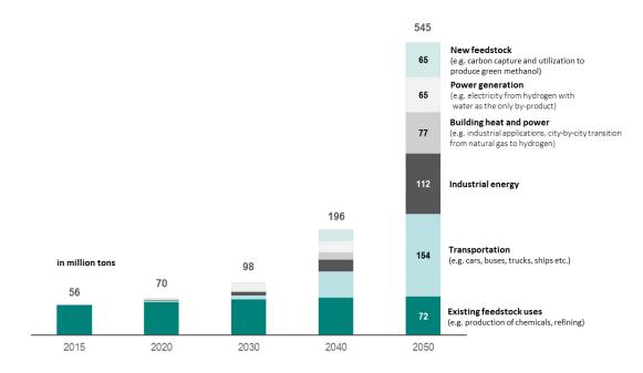
Figure 1. Forecast of the hydrogen demand by sectors [1]
