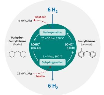
Figure 2. Hydrogen storage and release cycle of the LOHC technology
