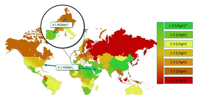
Figure 3. Cost differences for the regenerative generation of hydrogen [4],\*[5]
