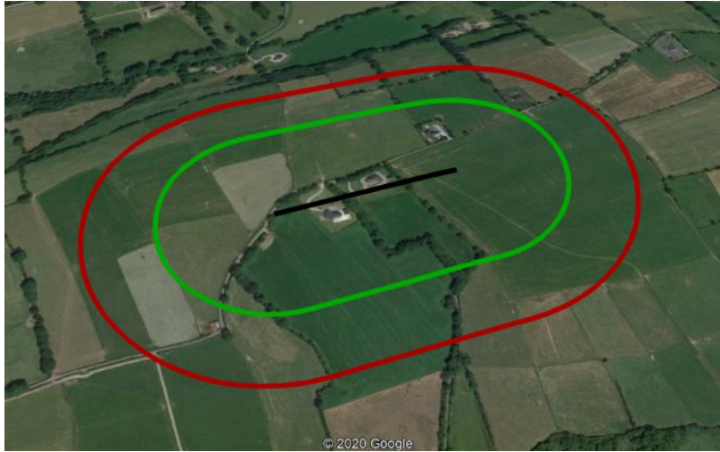
Figure 5 Standard Escape Distance – Methane (red) vs Hydrogen (green) (ID = 0.7m, 70 bar)
