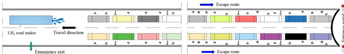
Figure 2. Layout of the vehicles in the queue upstream of the LH<sub>2</sub> road tanker for the tunnel tube investigated.
