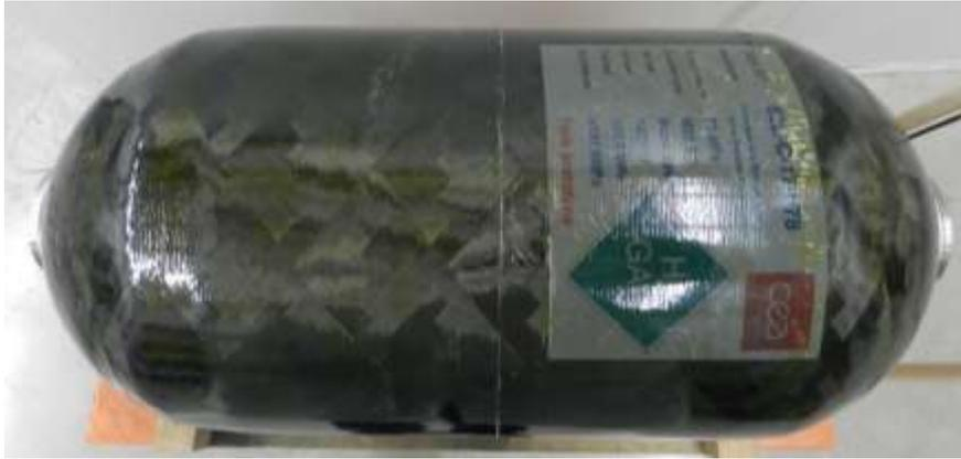
Figure 3. CEA 62L 700 bar Type IV H<sub>2</sub> Composite Pressure Vessel before burst test
