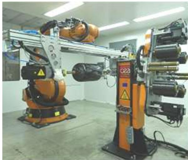
Figure 2. CEA Robotic Filament Winding Machine with On-board rotational delivery system
