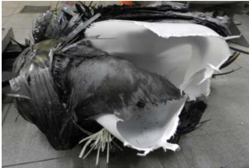
Figure 4. CEA 62L 700 bar Type IV H<sub>2</sub> Composite Pressure Vessel after 1800 bar burst test
