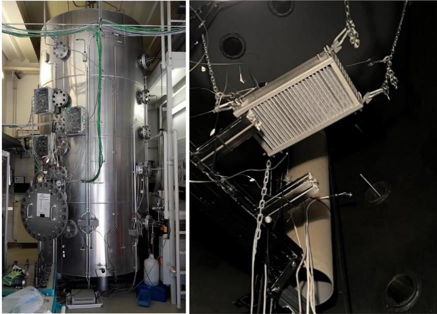
Figure 3. REKO-4 facility (left), PAR installation next to the mixing fan (right).
