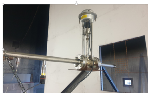
Figure 3: Nozzle rear view, pressure measurement instrumentation.
