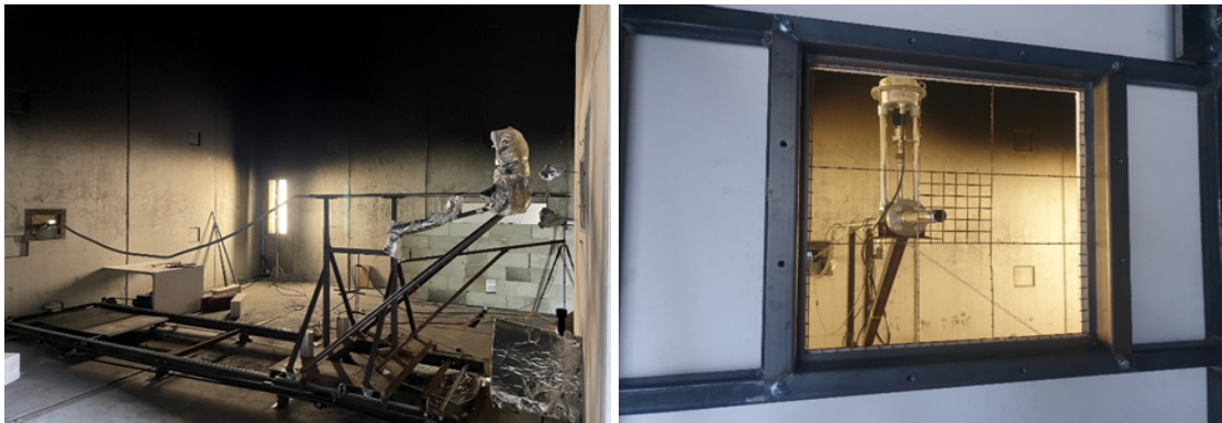
Figure 2: Visualization of the test facility. Left: moving bench, right: nozzle and temperature measurement grid.
