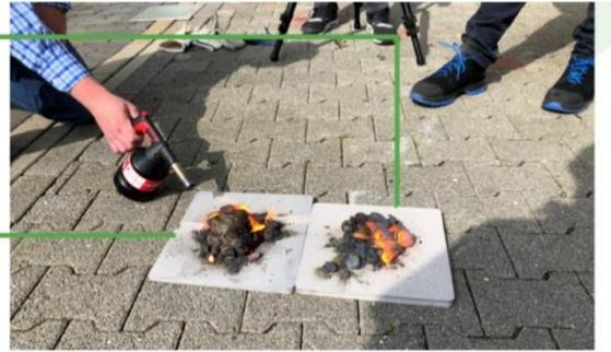
Figure 5. Heating of solid metal hydride blocks with a blowtorch for 2.5 and 4.5 minutes showing slow spread of flame front
