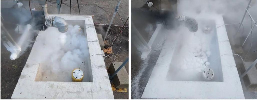
Figure 6: LH2 released into a concrete bund at 1.0 barg and from a height of 570 mm at the start of the experiment (left) and after all liquid H2 has evaporated showing a formation of solidied air (right).
