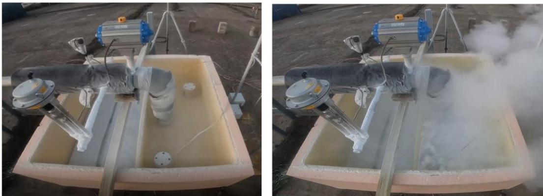
Figure 4: The image on the left shows an iso box used as a bund area for the LH2 pool; a coating of Chartek CSP has been applied to the inside of the box. The image on the right shows vapour dispersion from a quiescent pool of LH2 after filling has stopped.
