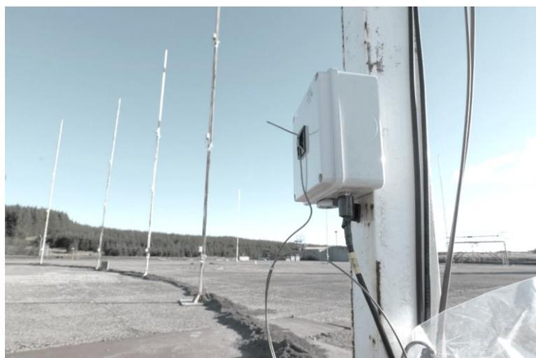
Figure 3: The instrument array installed along two arcs of five stands and at three heights. The box contains the oxygen depletion sensor and a Type T thermocouple is mounted on the front.
