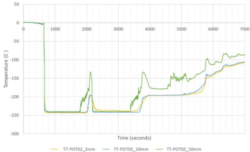
Figure 5: The temperature of the LH2 pool recorded by thermocouples at 2, 10 and 50 mm above the floor of the bund with a Chartek CSP system. The bund was filled at 625 s and then refilled at 2150 s.
