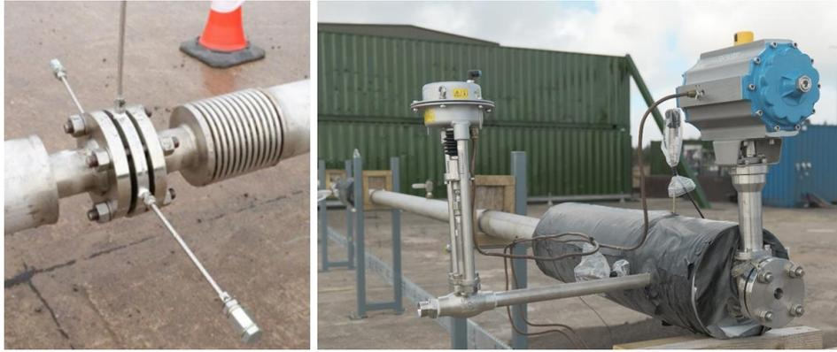
Figure 2: The image on the left shows the insulated pipework, spiral wound metaflex gasket and additional “flange” with temperature / pressure sensors. The image on the right shows the discharge line as it extends across the test pad from the iso-containers to the main valve and a 25 mm discharge orifice. A bypass valve is located to the left and before the final valve.
