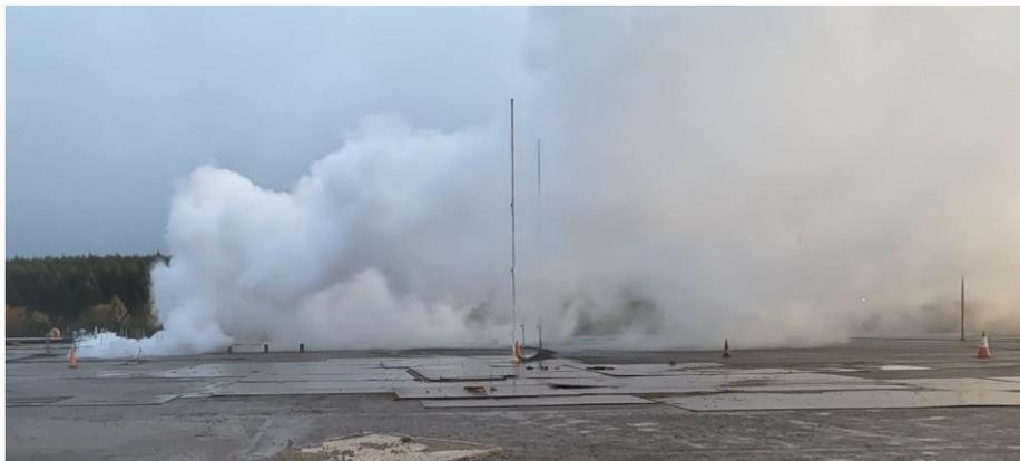
Figure 8: Dense gas dispersion from a quiescent pool of LH2 during Test 13.
