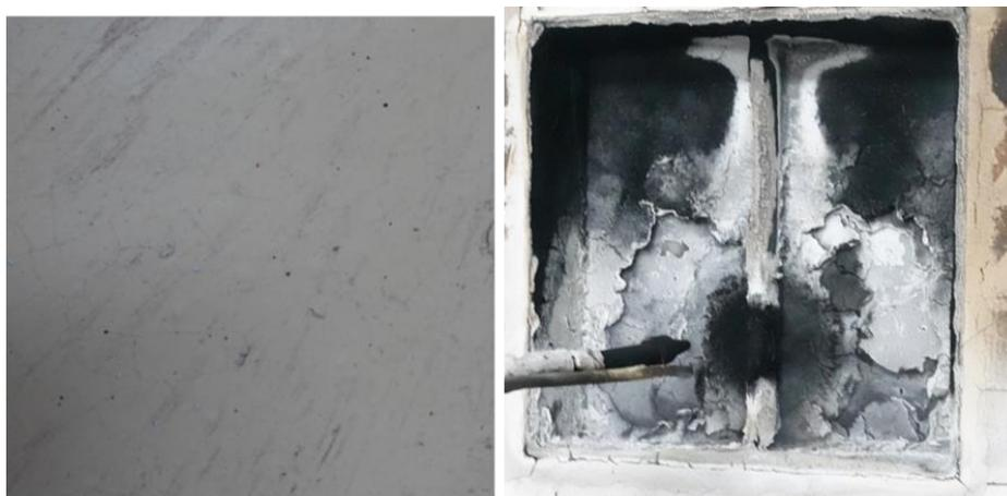
Figure 7: The Chartek CSP surface after exposure to LH2 (left) and following jet fire testing (right).
